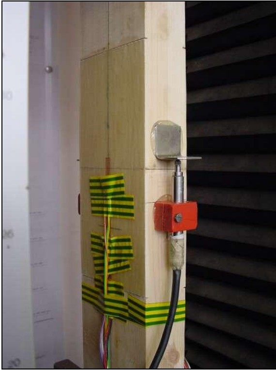
Figure 5 Sample in position ready for the fatigue test.
