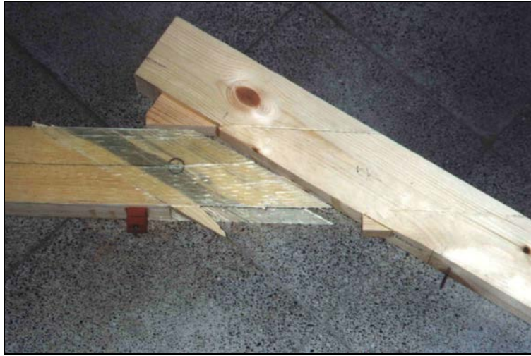
Figure 10. Top delamination on both sides at failure of TNU30 sample
