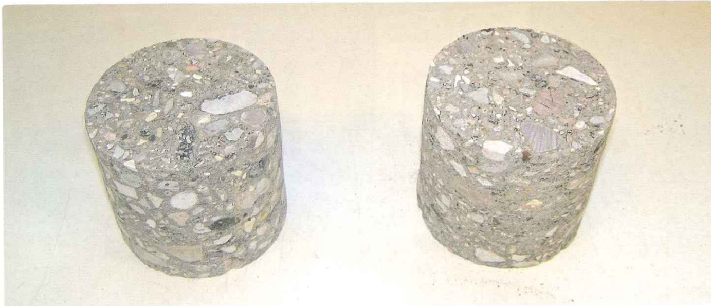
Figure 2: Cores from trial of roller-compacted concrete with CEM 0 and crushed concrete aggregate used in a car park.
