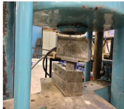
Figure 2 50mm cube compaction at 52kN
