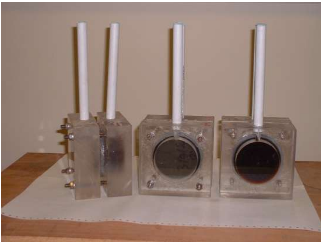
Fig.4.22 Diffusion cells used in this investigation.
