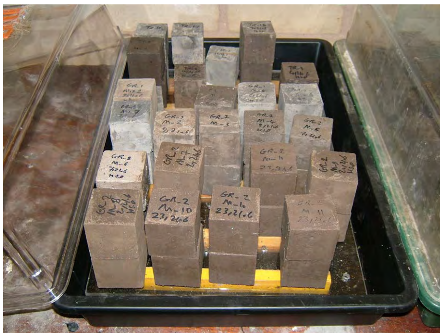
Figure B8 Paste samples stored in a container at 20 \pm 2^\circ \text{C} and 98% RH
