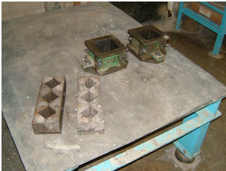
Figure B7 100 mm and 50 mm cube moulds, places and mechanical vibrator table
