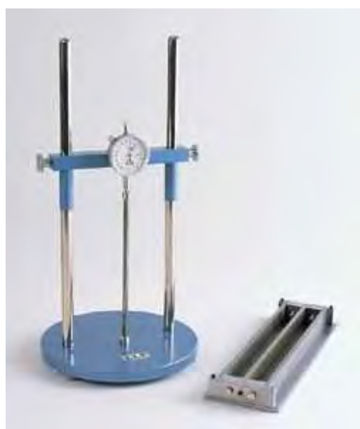
Figure 86 Apparatus for determination of length change
