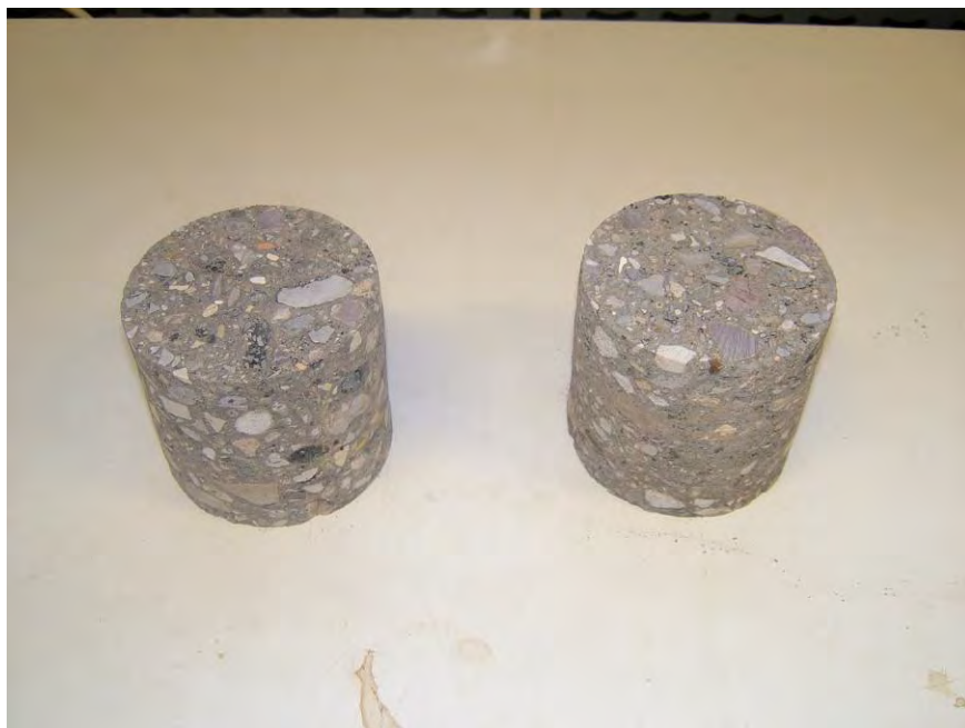
Figure 135 RCC core samples taken from different locations of the trial car park at the Lowdham Grange site
