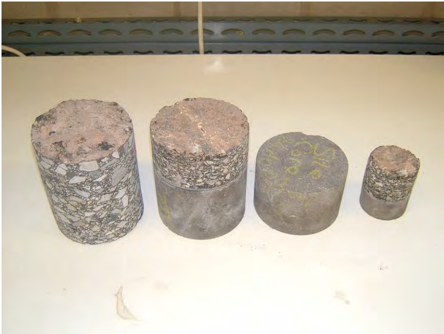
Figure 131 Core samples taken from different locations in the trial road at the King's Mill Hospital site
