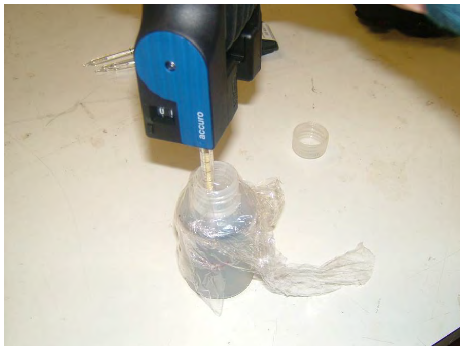
Figure 76 Testing the paste samples using the H 2 S detection tube
