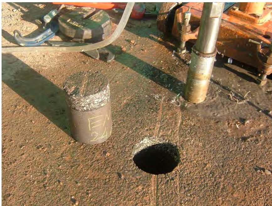
Figure 130 Core sample taken from the lower part of trial road at the King's Mill Hospital site
