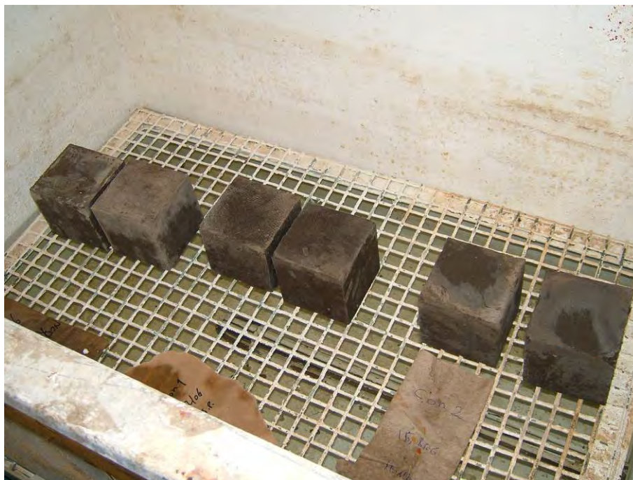
Figure B9 Concrete samples stored in a tank at 20 \pm 2^\circ \text{C} and 98% RH
