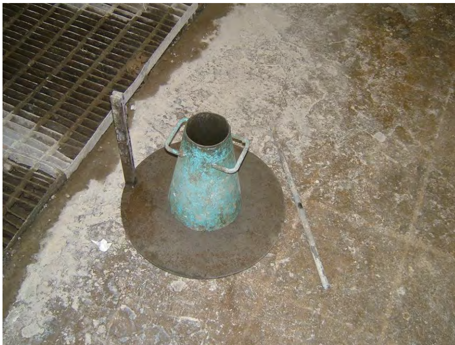
Figure B4 Slump test truncate cone and base
