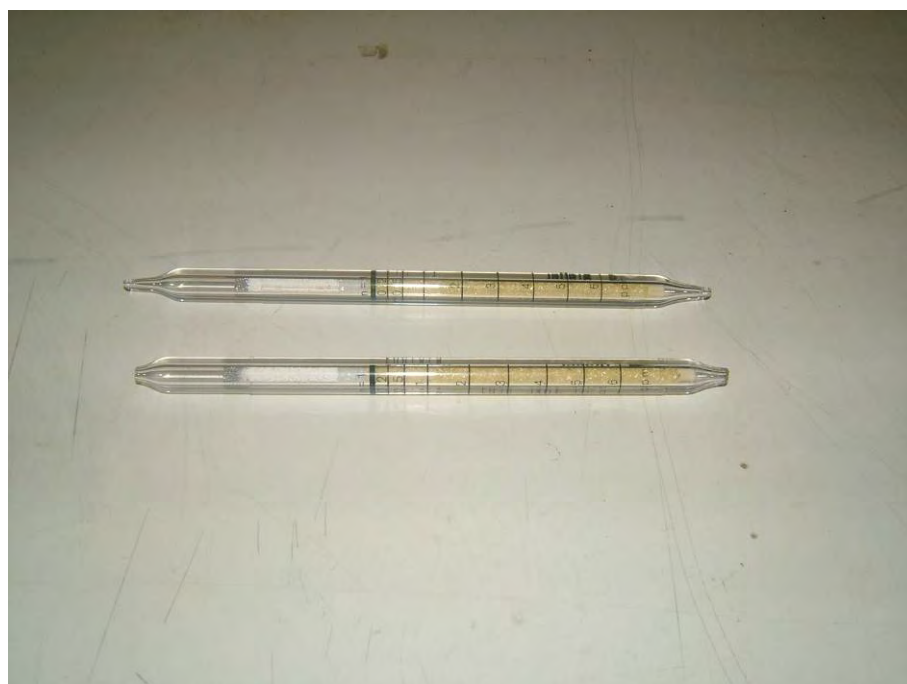
Figure 77 Comparison between new and used H 2 S detection tube for mix containing 50% paper
