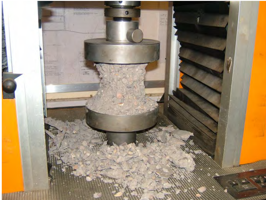
Figure B14 A concrete sample after crushing
