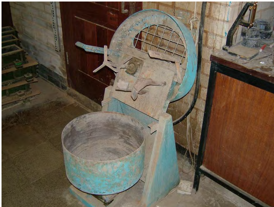
Figure B2 Pan mixer used to make concrete mixes
