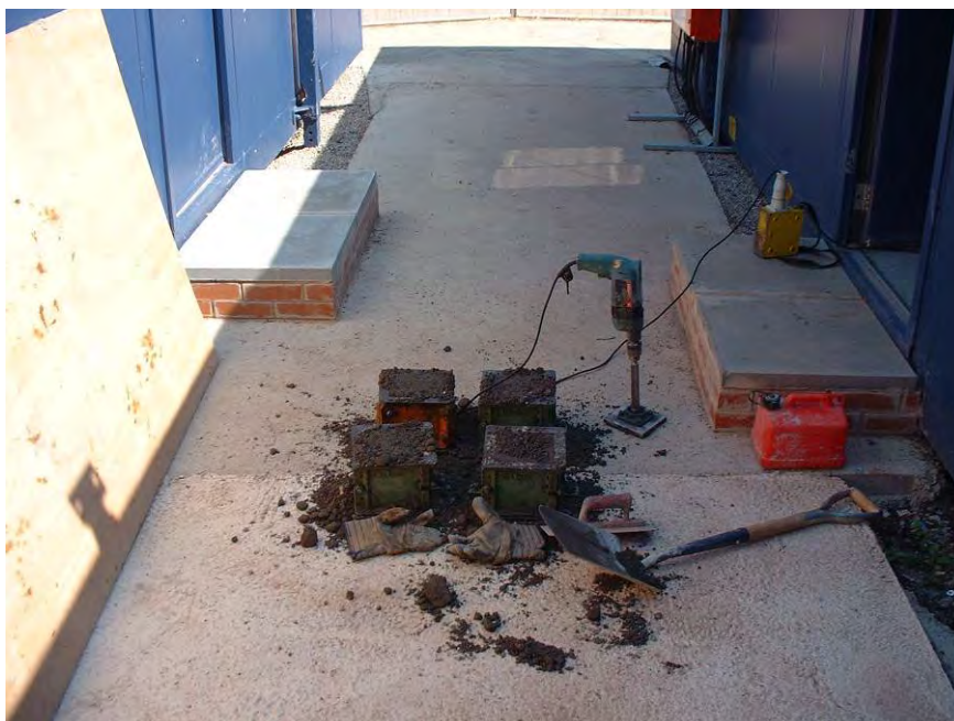
Figure 103 Sampling of concrete using 150-mm cubes and hammer drill
