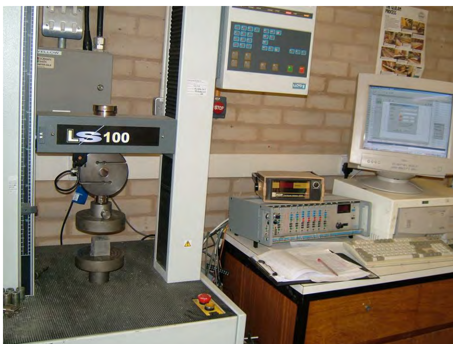
Figure B10 Computerised compressive strength testing machine for paste specimens
