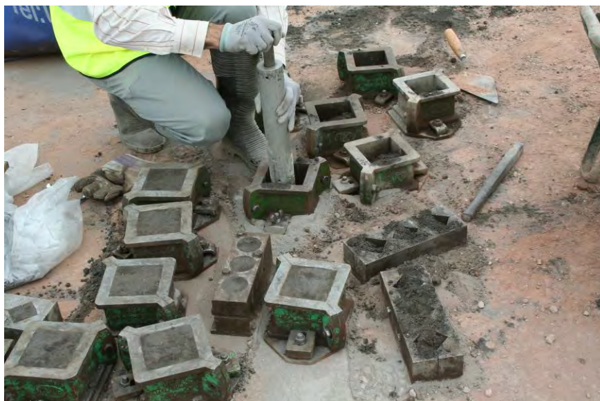
Figure 125 Sampling the semi-dry paste using 100 and 50 mm cubes
