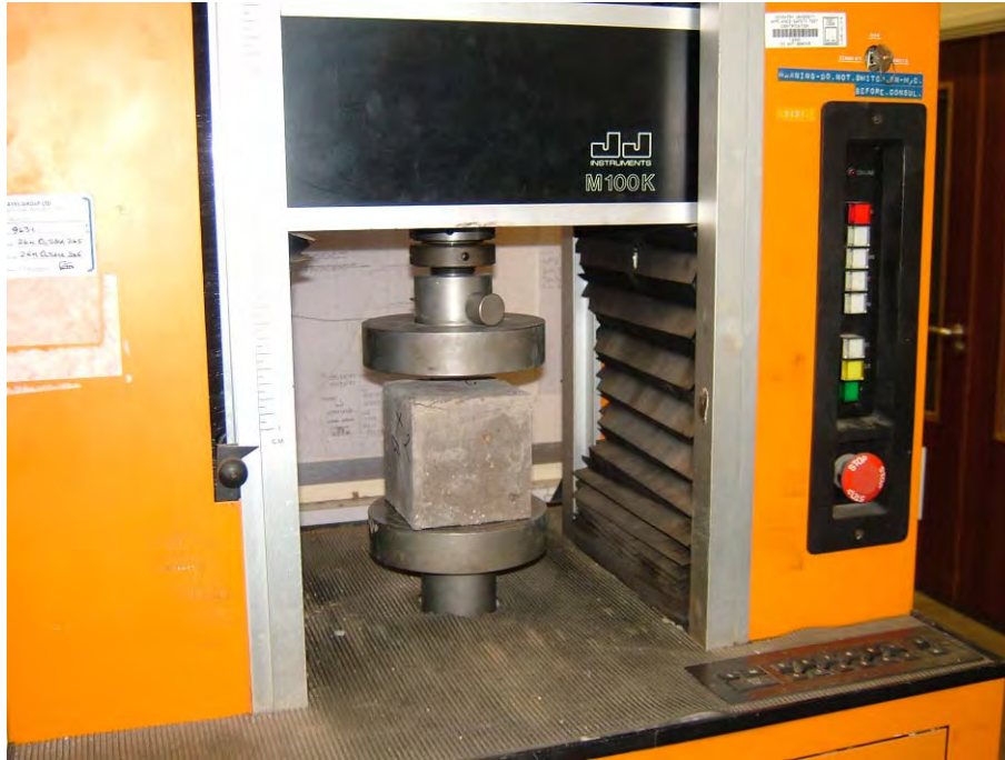
Figure B13 The 100 kN compressive strength testing machine for concrete specimens at early ages
