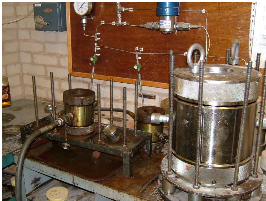
Figure 78 Hoek cells used for high pressure through-flow test
