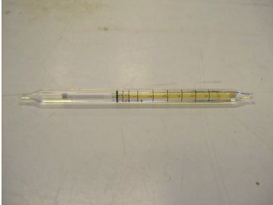
Figure 74 Drager Accuro H_2S detection tube
