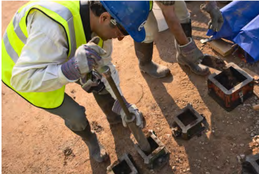
Figure 119 Sampling the stabilised soil
