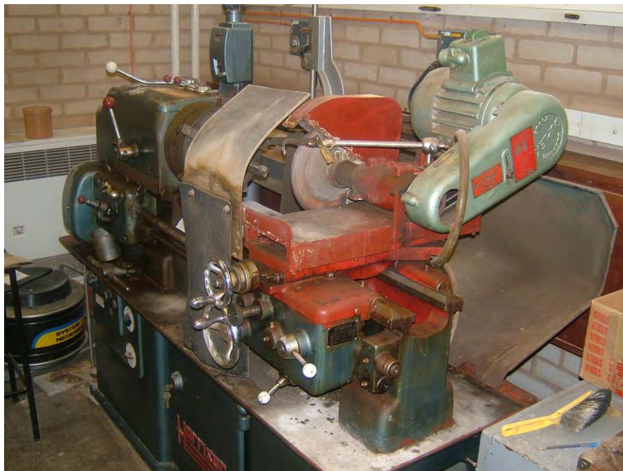
Figure B15 Special cutting machine for concrete samples (built from lathe)
