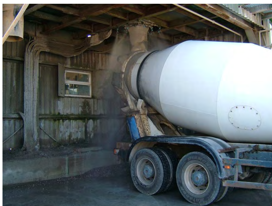
Figure 95 Loading aggregates and water into the truck mixer
