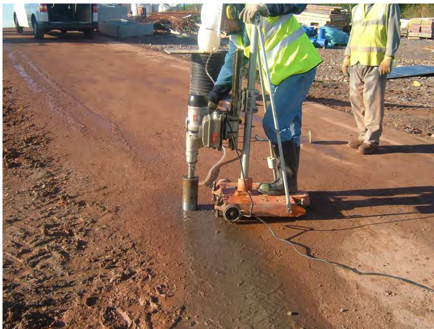
Figure 129 Coring machine used to drill the cores at the King's Mill Hospital site
