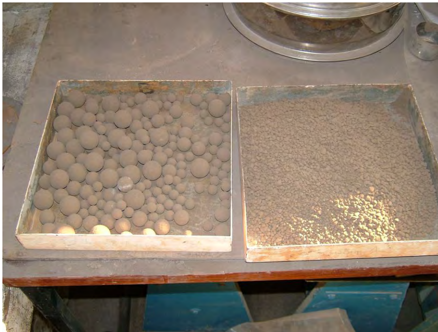
Figure B6 Metallic balls of different sizes used in the ball mill to grind the slag
