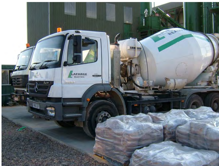
Figure 90 Blended powder delivered to the ready-mix plant in 20-kg bags
