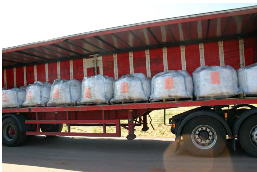
Figure 91 Blended powder delivered to the King's Mill Hospital site in 1000-kg sling bags
