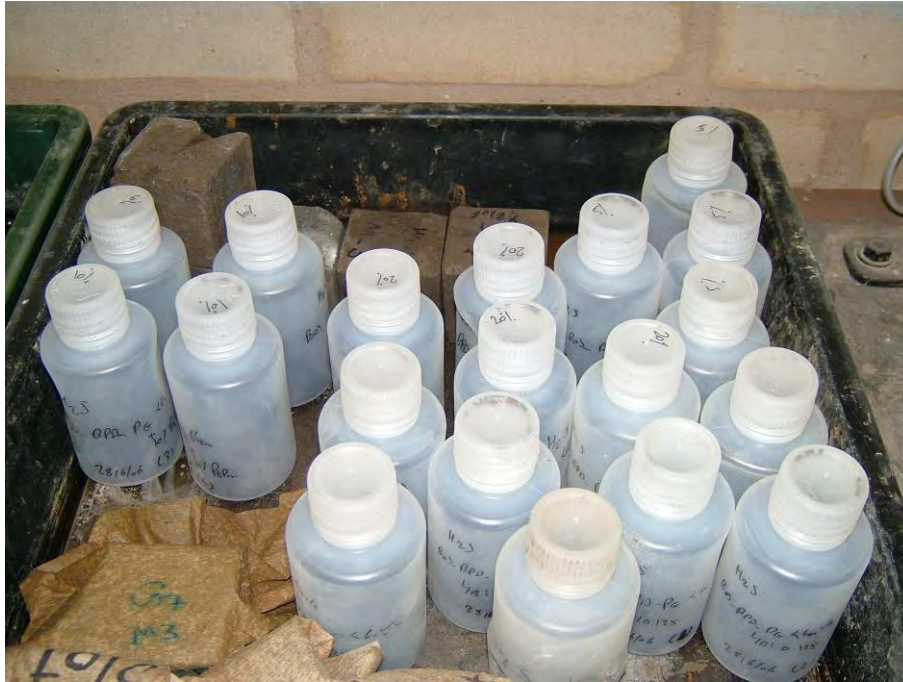
Figure 68 Plastic bottles containing paste specimens for H_2S check
