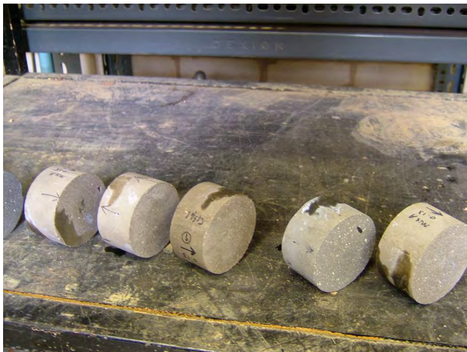
Figure 79 Paste specimens prepared for high pressure through-flow test
