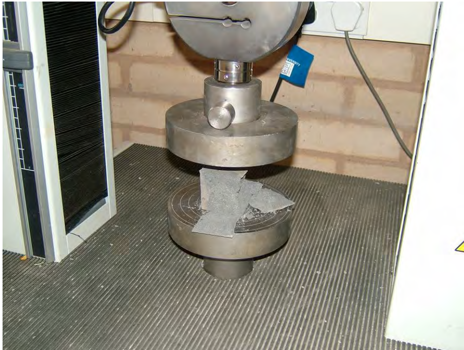
Figure B12 A paste sample after crushing
