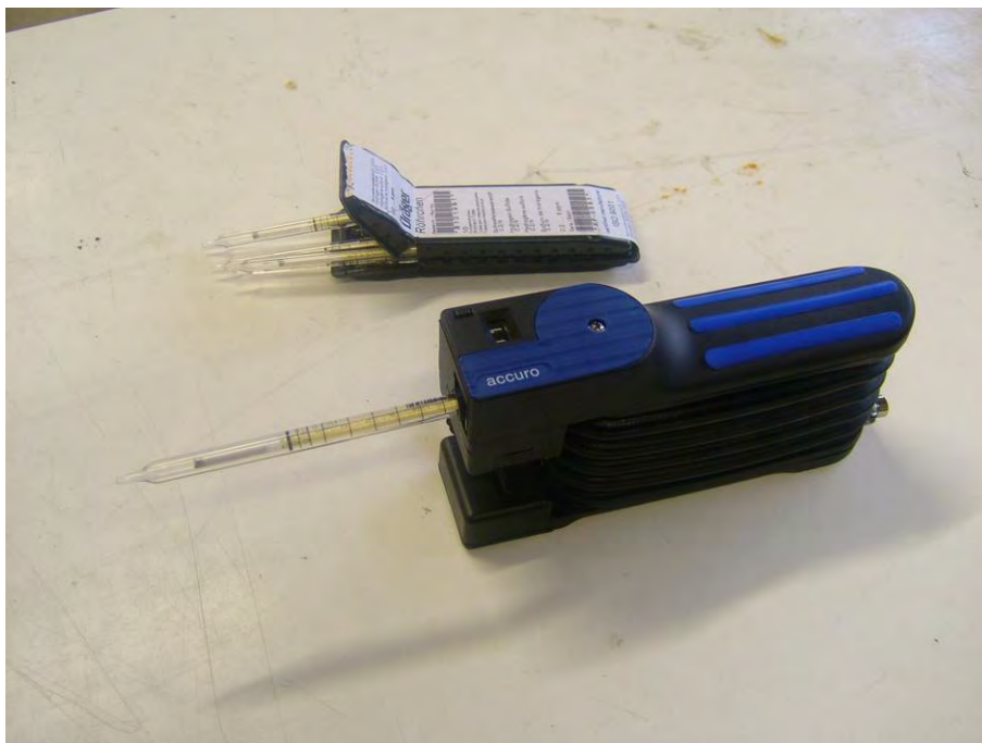
Figure 75 Drager Accuro pump kit and H_2S detection tube
