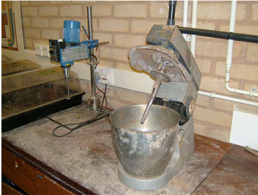
Figure B1 Small mixers used to make 'cup' mixes and main paste mixes
