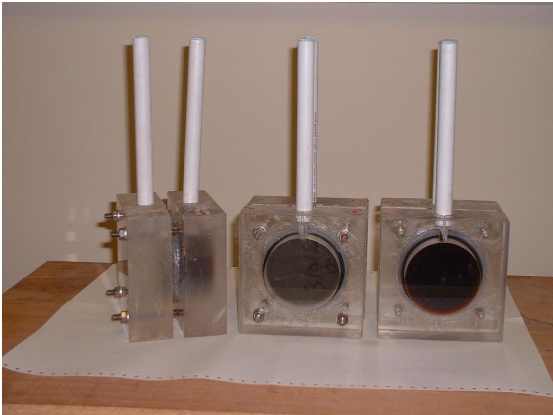
Figure 1: The new composite landfill liner.
