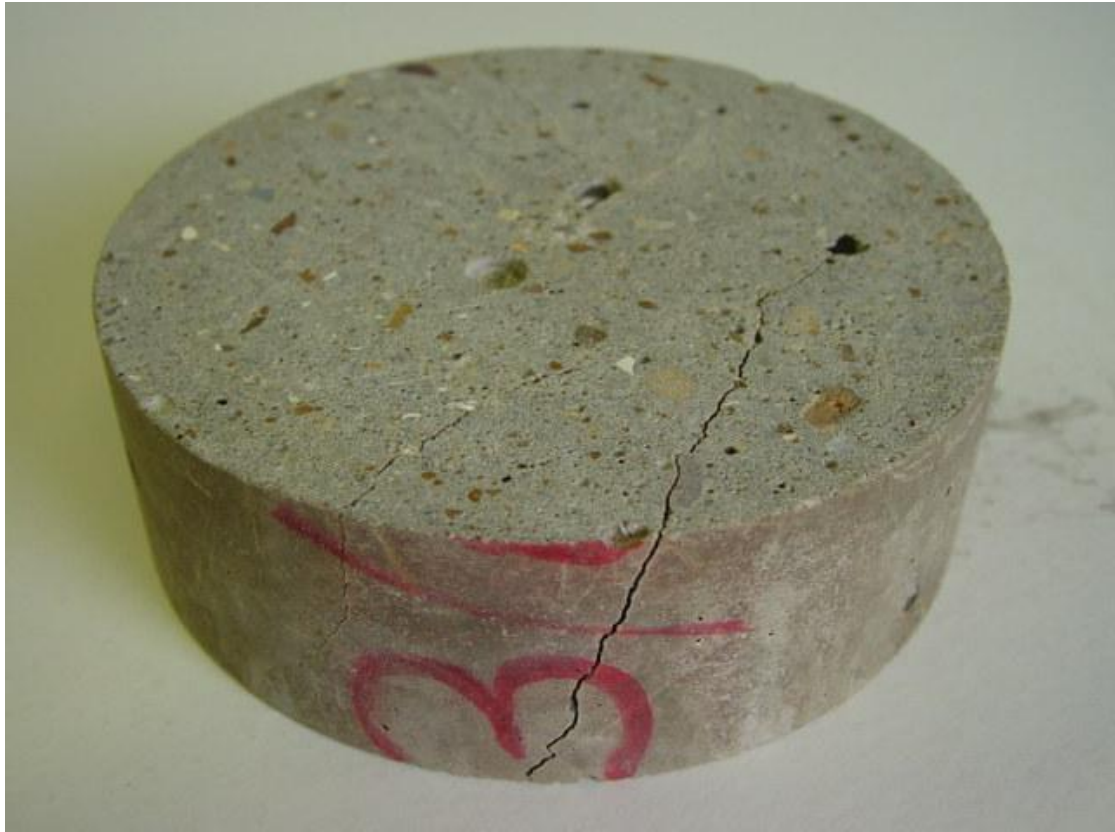
Fig. 5: Narrow cracks induced in the F.R. mortar disc.
