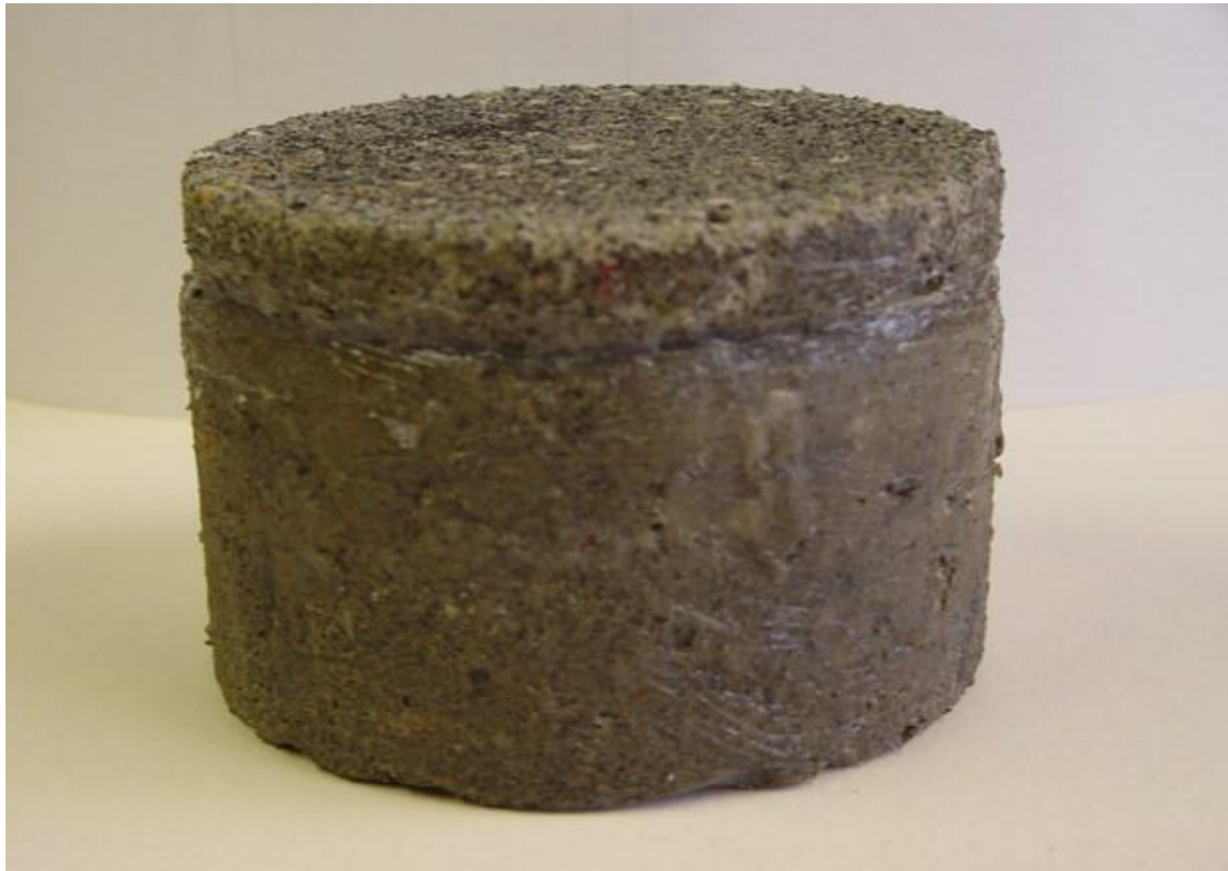
Fig. 8: Multi layer sample with partially compacted clay inside it.
