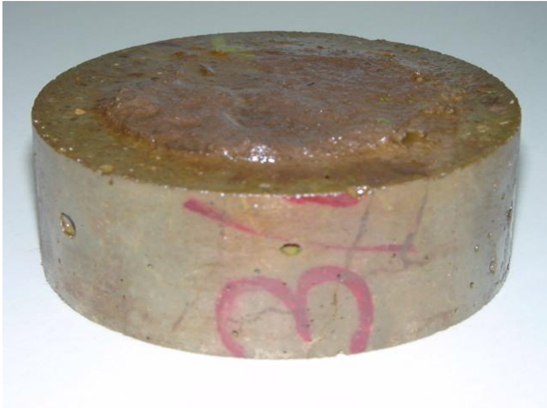
Fig. 6: Cracked sample after clay has sealed the cracks.
