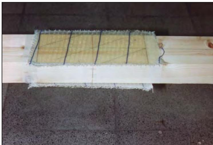
*Figure4.35 The layer of glass fibre is bonded onto the other side.*
