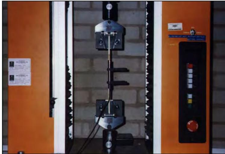
*Figure 4.54 Tension parallel to the grain test configuration.*
