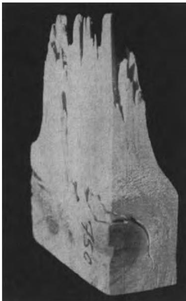
*Figure 3.4 Tension failure of a spruce board cause by fibre inclination around a knot (Hoffmeyer, in Timber Eng. STEP1, 1995).*
