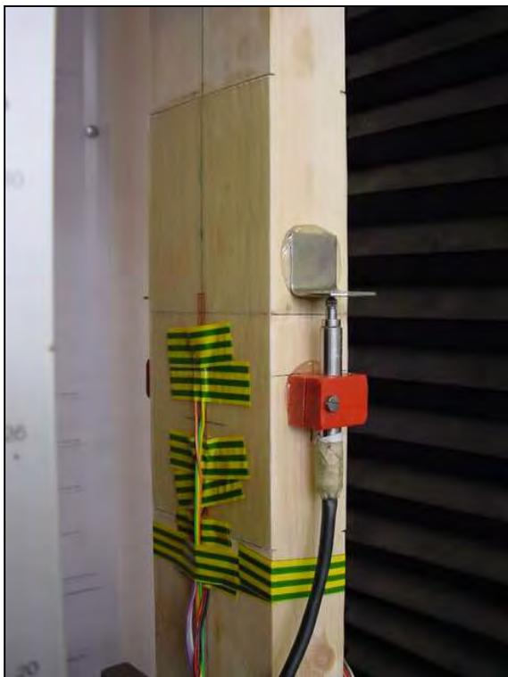
*Figure 7.7 Sample in position ready for the fatigue test.*
