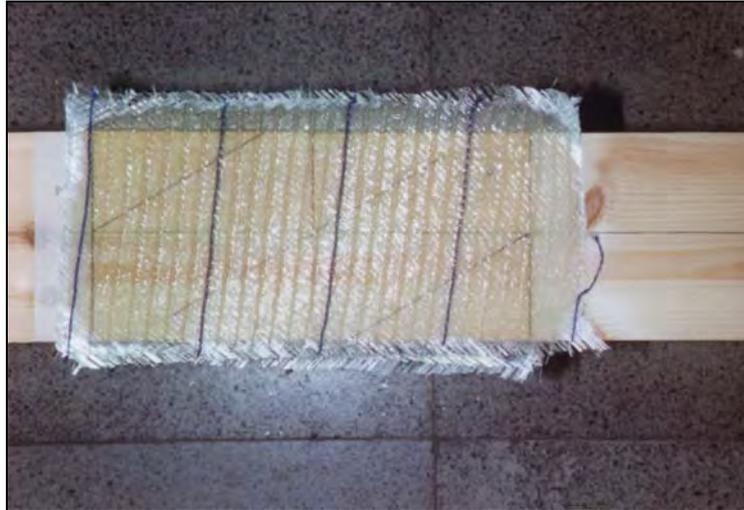
*Figure 4.34 The first layer of glass fibre is bonded on the timber.*
