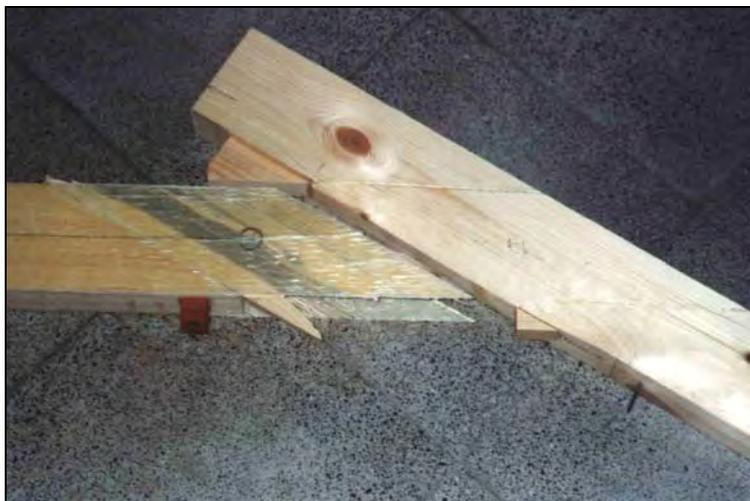
*Figure 5.19 Top delamination on both sides at failure of sample 4TNU30 - X.*
