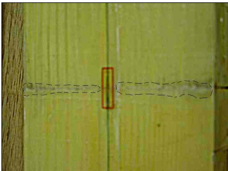
*Figure 7.35 Visible damage in the gap zone of the composite layer after the fatigue test.*
