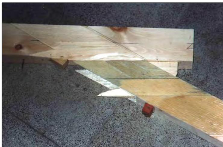
*Figure 5.20 Top delamination on both sides at failure of sample 5TNU30 - Z.*
