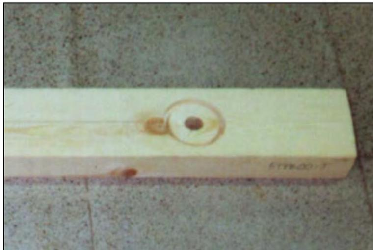
*Figure 4.31 Drilling of each timber piece end for shear plate connector.*
