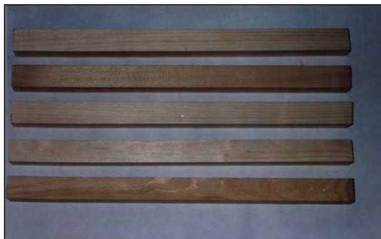
*Figure 4.49 Static bending test samples.*
