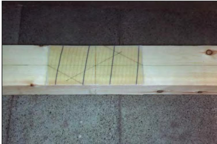
*4.36 Sample with composite excess removed.*
