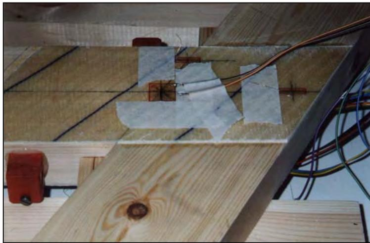
*Figure 4.46 Strain gauges and soldered to cables and isolated with craft tape.*
