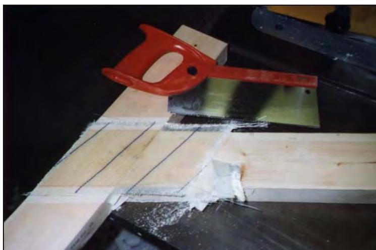
*Figure 4.42 A handsaw is used to remove the excess of composite.*
