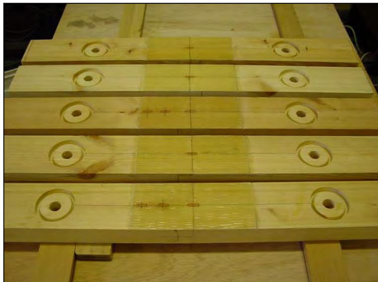
*Figure 7.6 Strain gauges positions on fatigue test samples.*
