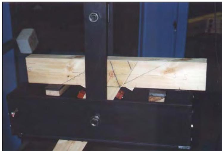
*Figure 4.26 Sample configuration when positioned within the steel box.*
