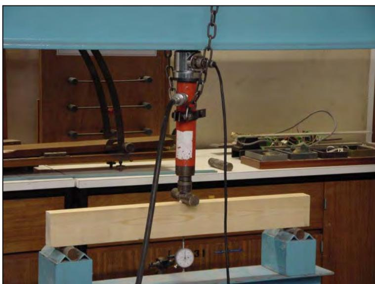
*Figure 7.8 Three points bending test of one timber plank before joint fabrication.*
