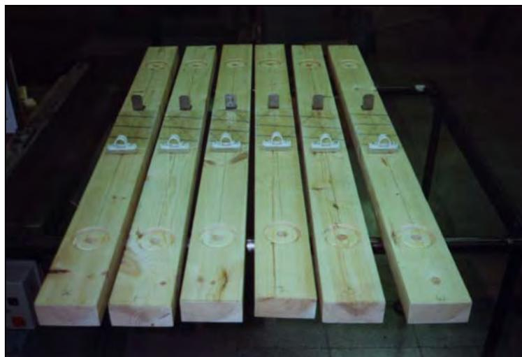
*Figure 4.37 Brackets are fixed onto the samples.*
