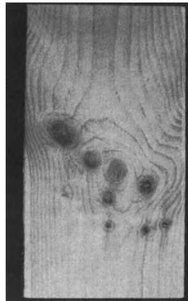
*Figure 3.5 A softwood board may show knots in clusters separated by the often clear wood of the inter-nodes (Hoffmeyer, in Timber Eng. STEP1, 1995).*
