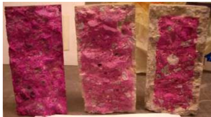
Figure 4. Depth of carbonation of concrete mixtures containing 35% fly ash, measured at 28 days.
