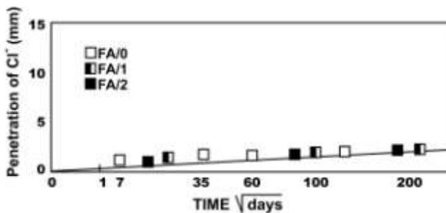
Figure 9. Penetration of Cl<sup>-</sup> ions as a function of time ( $\sqrt{t}$ ) in SCCs with fly ash and UFACS (Table 4).
