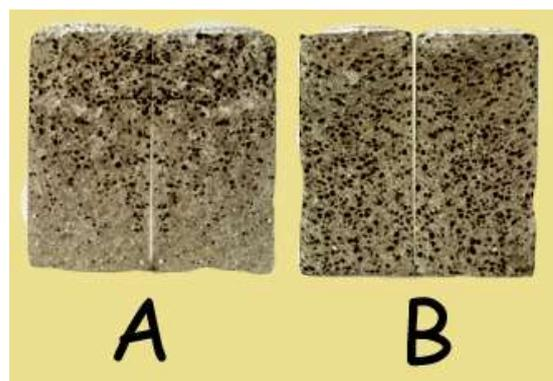
Figure 11. Flowing concrete with segregation of the lightweight coarse aggregate on the top (A) in comparison with the corresponding lightweight SCC without segregation.
