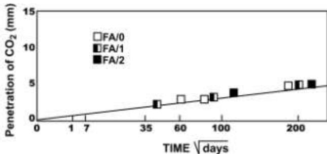
Figure 8 – Penetration of CO<sub>2</sub> as a function of time ( $\sqrt{t}$ ) in SCCs with fly ash and UFACS (Table 4).
