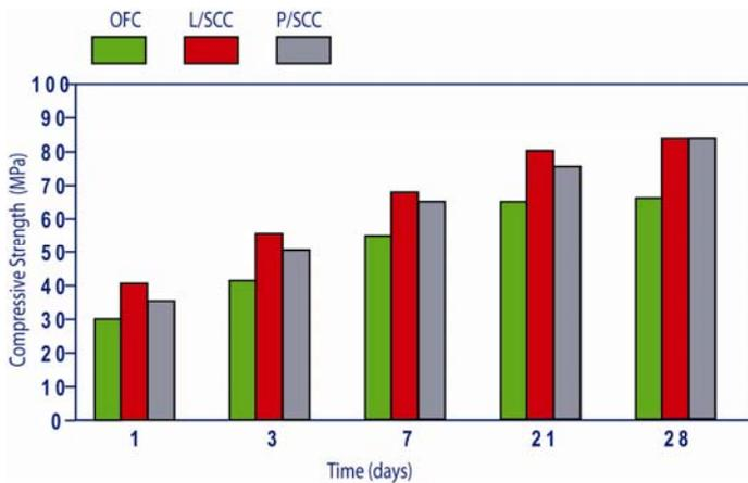
Figure 4. Compressive Strength of OFC, L/SCC and F/SCC.
