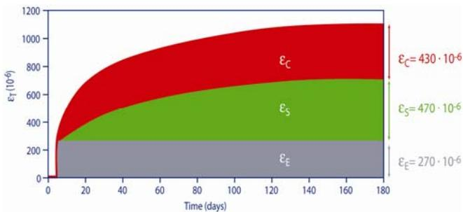
Figure 12. OFC: elastic strain ( $\epsilon_E$ ), drying-shrinkage ( $\epsilon_S$ ) and creep strain ( $\epsilon_C$ ) at R.H. of 65% with a load of 163 MPa at 7 days (1/4 of 65 MPa).
