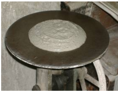
Photograph 4. Device for flow test
