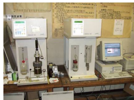
Photograph 7. Device for mercury intrusion porosimetry
