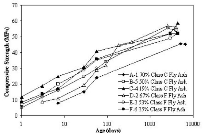
Fig. 4. Compressive Strength of Concrete Pavements (using cores after 365 days) [Naik et al. 2004]
