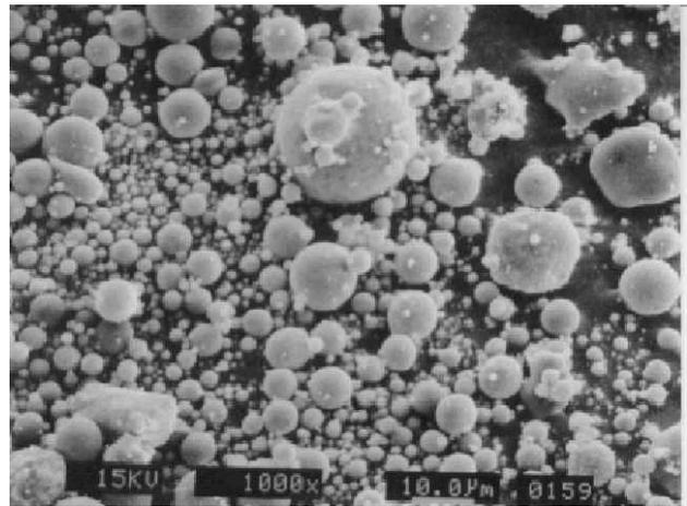
Fig. 1. Scanning electron micrograph of fly ash particles.
