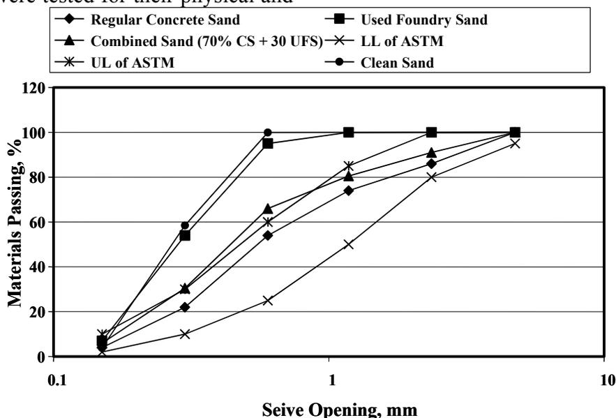
Fig. 6. Gradation of concrete sand, clean foundry sand, and used foundry sand (ASTM C 136) [Naik et al. 2001]
