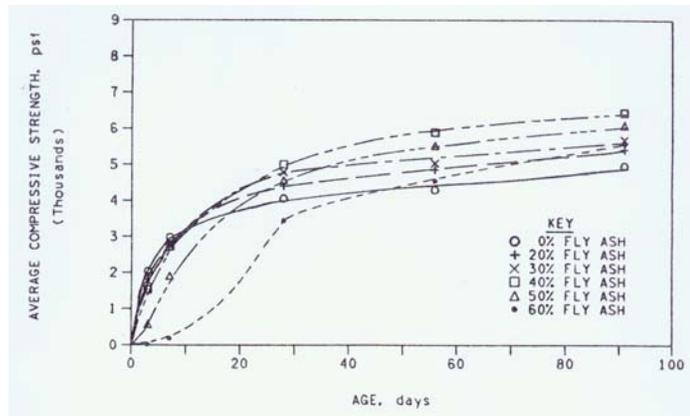
Fig. 2 – Concrete Mixtures Using Class C Fly Ash – 28-day Design Strength of 21 MPa (3,000psi) [Naik & Ramme 1989]
