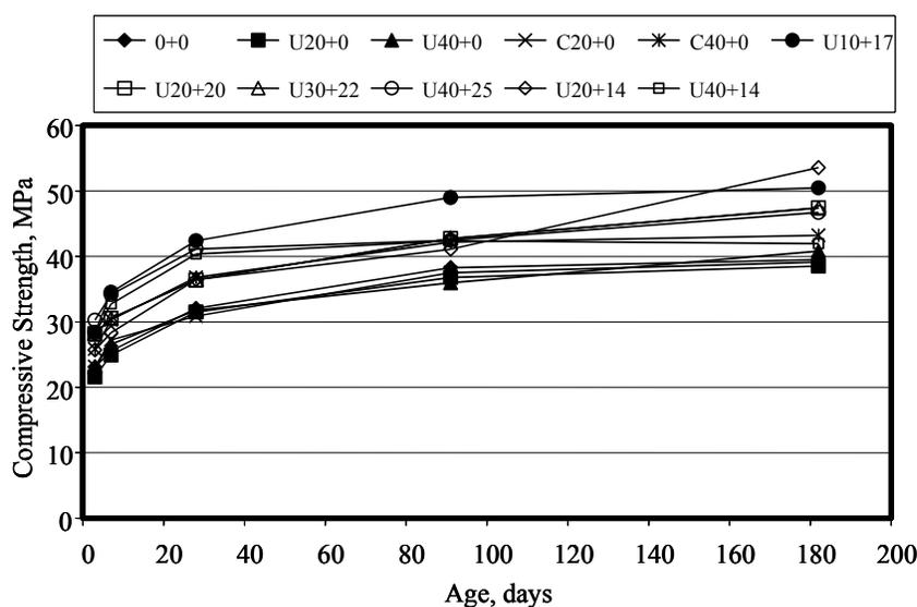
Fig. 7. Compressive strength of concrete mixtures using foundry sand [Naik et al. 2001]
