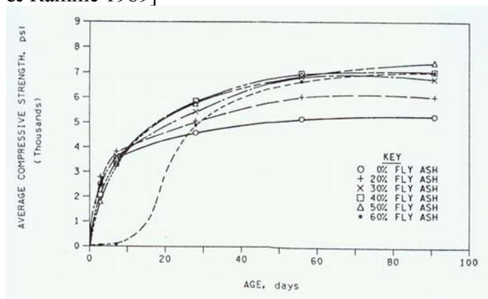
Fig. 3. Concrete Mixtures Using Class C Fly Ash – 28-day Design Strength of 28 MPa (4,000psi) [Naik & Ramme 1989].
