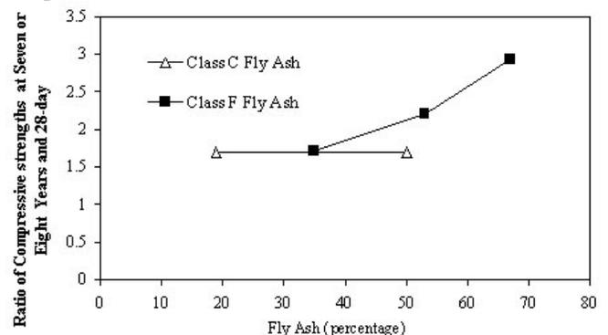
Fig. 5 – Rate of Strength Gain for Concrete Using Class C and Class F Fly Ash [Naik et al. 2004]
