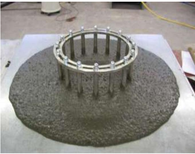
Figure 3. J-ring test of SCLC
