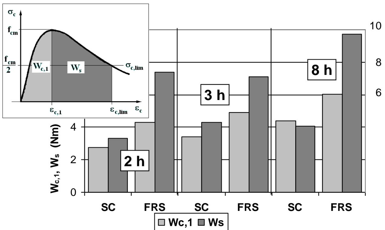
Figure 9. Average values of absorptive energies  $W_{c,1}$  and  $W_s$  of SC and FRS at ages 2,3 and 8 hours.
