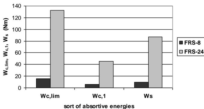
Figure 11. Average values of absorptive energies  $W_{c,lim}$ ,  $W_s$  and  $W_{c,1}$  of 8 and 24-hours-old FRS.
