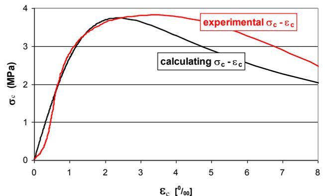
Figure 3. Experimental and calculating stress – strain diagrams of 7-hour-old FRS.
