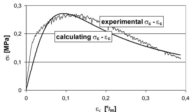
Figure 6. Experimental and calculating stress – strain diagrams of 8-hour-old FRS.
