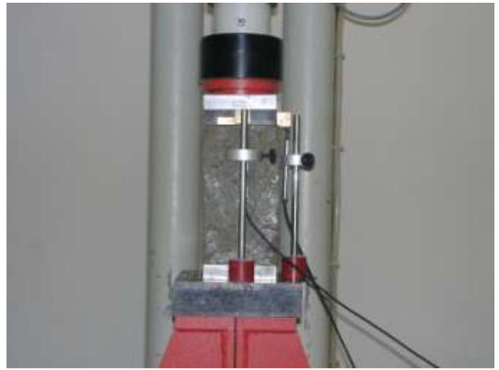
Figure 4. Test configuration for prism of  $100 \times 100 \times 200 \text{ mm}^3$ .
