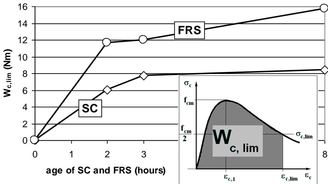
Figure 8. Average results of absorptive energy  $W_{c,lim}$  of SC and FRS at ages of 2, 3 and 8 hours.
