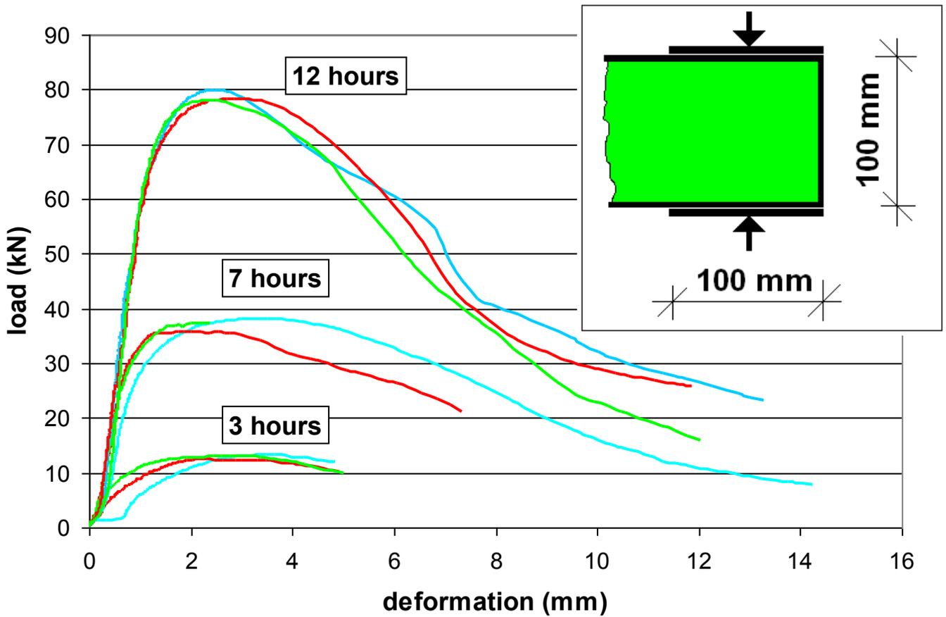
Figure 2. Compressive load – deformation diagrams of FRS at the ages of 3, 7 and 12 hours.
