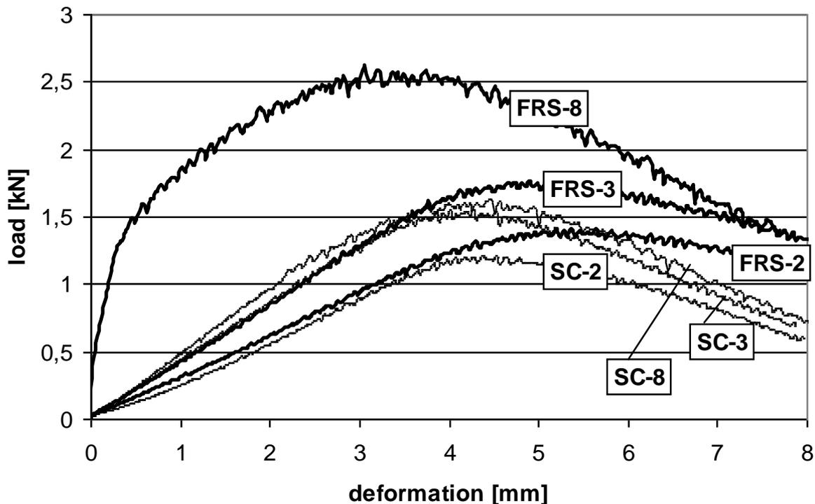
Figure 5. Characteristic load – deformation diagrams of SC and FRS at ages of 2 hours (SC-2, FRS-2), 3 hours (SC-3, FRS-3) and 8 hours (SC-8 and FRS-8).
