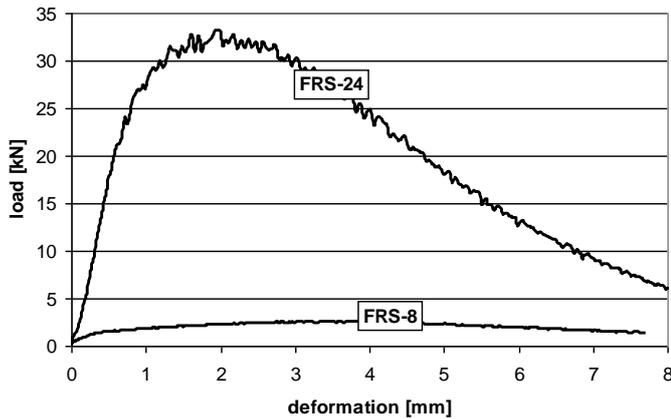
Figure 10. Characteristic load – deformation diagrams of FRS at age of 8 hours (FRS-8) and at age of 24 hours (FRS-24).
