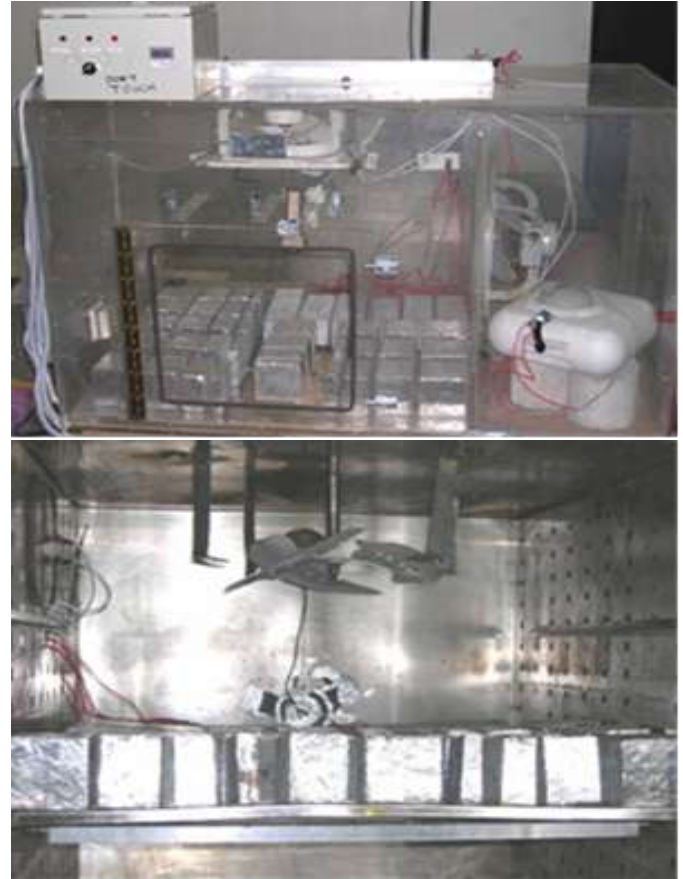
Figure 1. Pyrex glass (low wind) and steel (high wind) environmental chambers with drying specimens.
