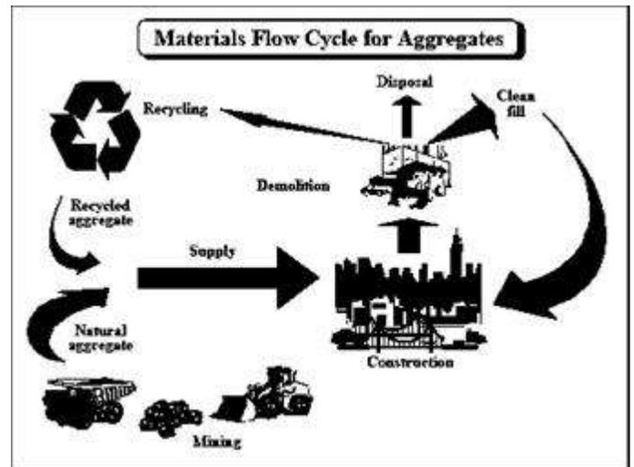
Figure 3. Aggregate material flow cycle
