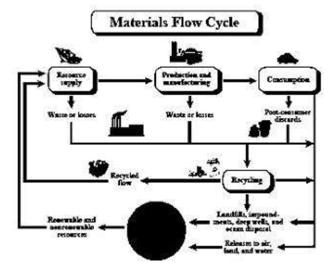
Figure 2. Overall material flow cycle
